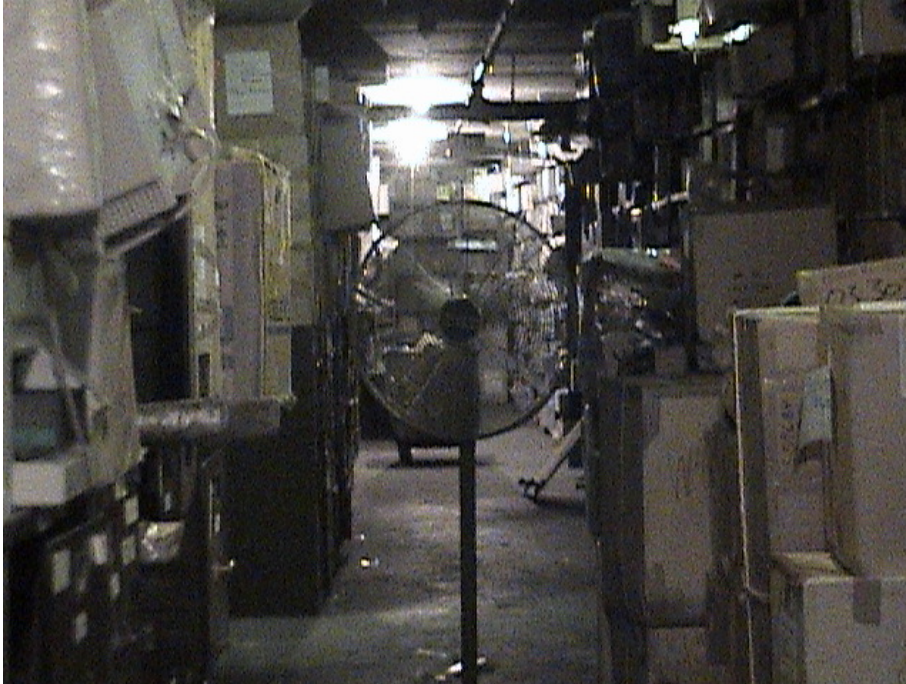
Figure I. Portable Fan Used to Circulate Air in Warehouse
